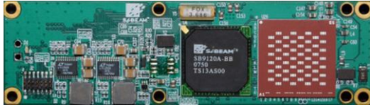
Figure 4 Typical reference design. Center chip is the digital baseband/MAC and the chip on the right side is the RF chip with integrated antennas. Other components include minor support circuitry such as voltage regulation and a frequency reference crystal. Actual size is approximately 12 by 3 cm.
